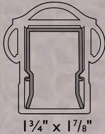
Unique full length PVC inserts in both the top and bottom rails to allow a faster, "screwless" assembly and create a tight, quiet fit.
