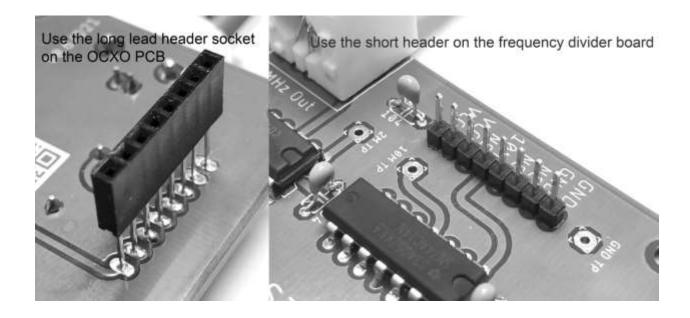
Use the above picture to understand how to use the headers to connect the boards electrically.
