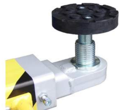
Double Telescoping Swivel Pads with 2-3/8" Height Adjustment
