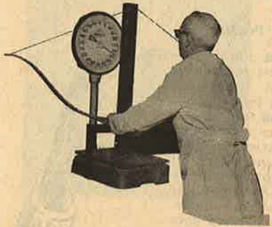
Herter precision machine for testing bow pull weight. Guaranteed actual weight.
