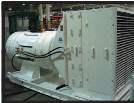
Engart 36,000 cfm skid mounted portable dust extractor unit
