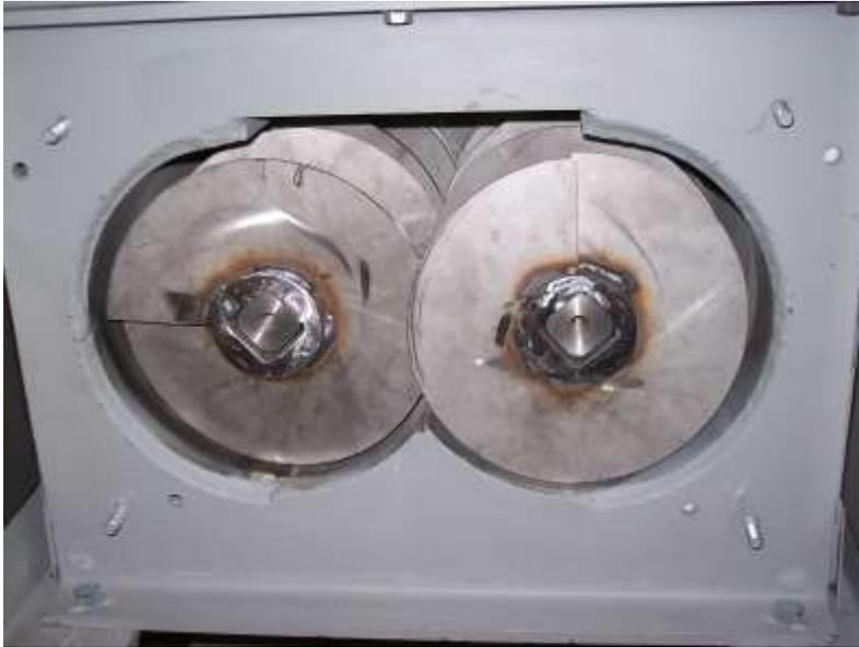
Edges of shafts should be in this position when removing and installing augers
