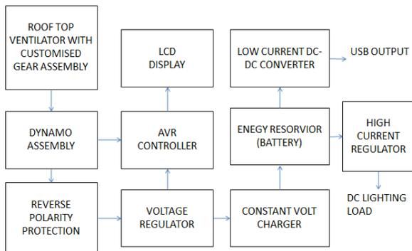
Fig.9: Block diagram
