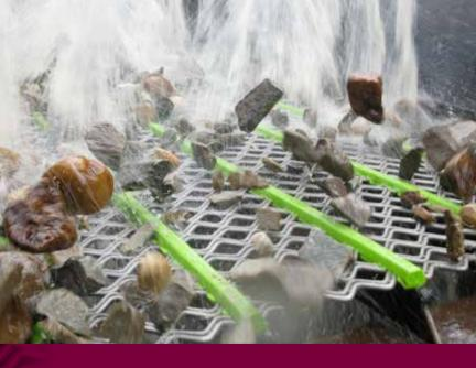
individual non-woven wires to maintain tight specifications while allowing them to vibrate independently at different frequencies.
