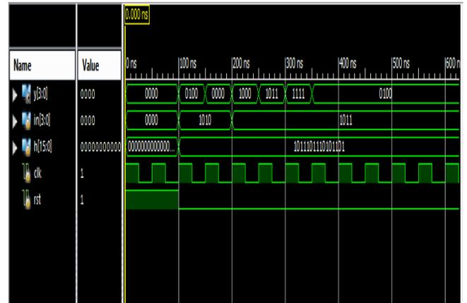
Fig.8: Fir filter with Wallace tree multiplier results
