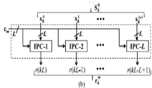
Fig.3: (a) Internal structure of RU for block size  $L = 4$ . (b) Structure of  $(m + 1)$ th IPU.
