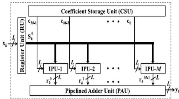
Fig.2: Proposed structure for block FIR filter.
