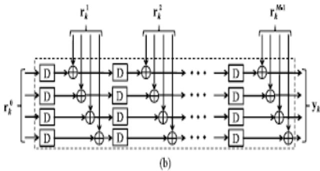
Fig.4: (a) Internal structure of  $(l + 1)$ th IPC for  $L = 4$ . (b) Structure of PAU for block size  $L = 4$ .
