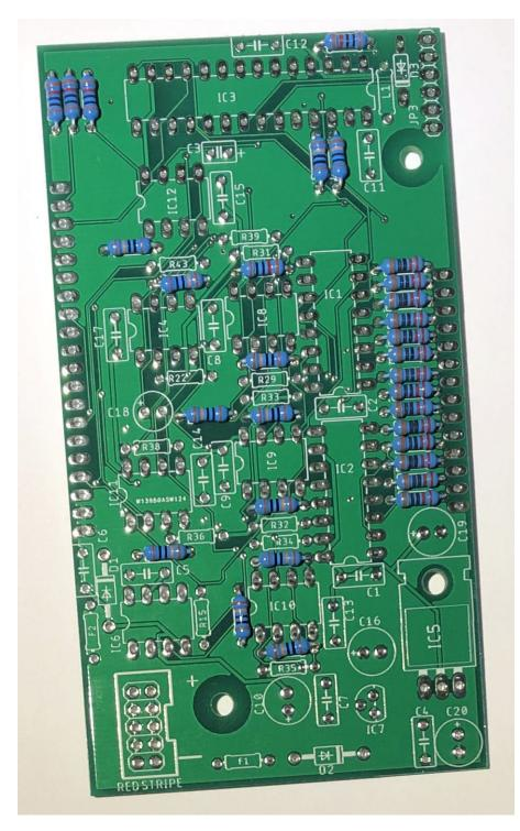
Install and solder the seven 150K resistors R29, R31, R32, R33, R34, R35 and R39
