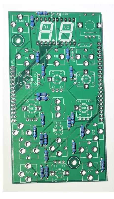
Install and solder C1 and L1
