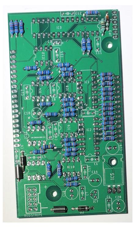
Cut the IC socket strips to the correct sizes. Start with the larger ones first to ensure there will be enough length remaining. Once all are cut to the correct sizes, install them and solder into place. Use a piece of cardboard, book etc to hold them in place while flipping the PCB over to solder.
