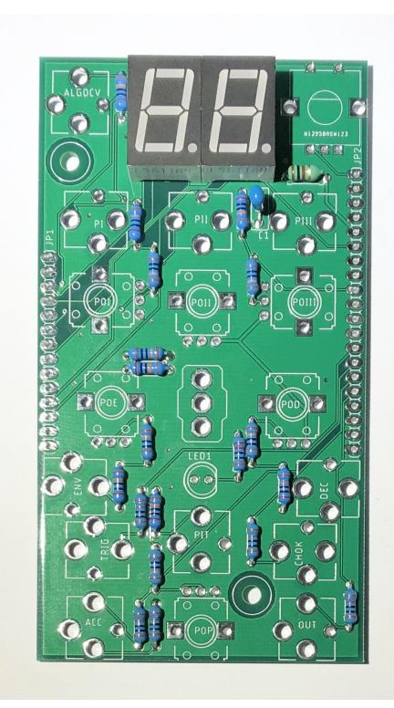
Cut the male header pin strip to size and solder in place, making sure it is at right angle to the PCB
