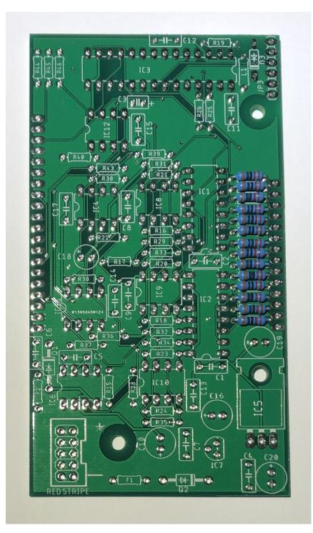
Install and solder the five 10K resistors R19, R21, R44, R45 and R46
