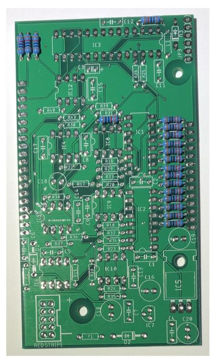
Install and solder the twelve 100K resistors R16, R17, R18, R20, R23, R24, R25, R26, R28, R30, R37 and R40
