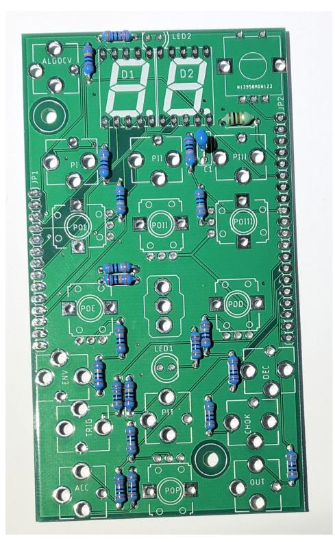
Install and solder the two seven segment displays D1 and D2
