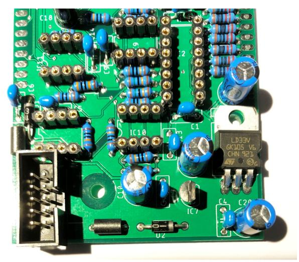
Cut a 1x6 piece of male pin header and install it into JP3 – this can be used to connect a PicKit3 programmer for firmware updates.
