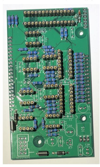
Install the fourteen 100nf COG capacitors C1, C2, C3, C4, C5, C6, C7, C8, C9, C11, C12, C13, C14, C15 and C17. Also install the LD1117V33 voltage regulator.
