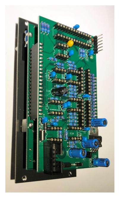
Now install the IC's paying VERY close attention to the orientation. Start with IC6 which is the TL071 as it is different to the rest. Next install the six MCP 602's, followed by the two 74HC595's and lastly the dsPIC microcontroller.
