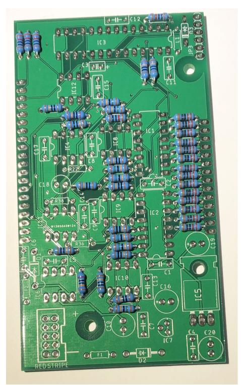
Install and solder the 300K resistor R36
