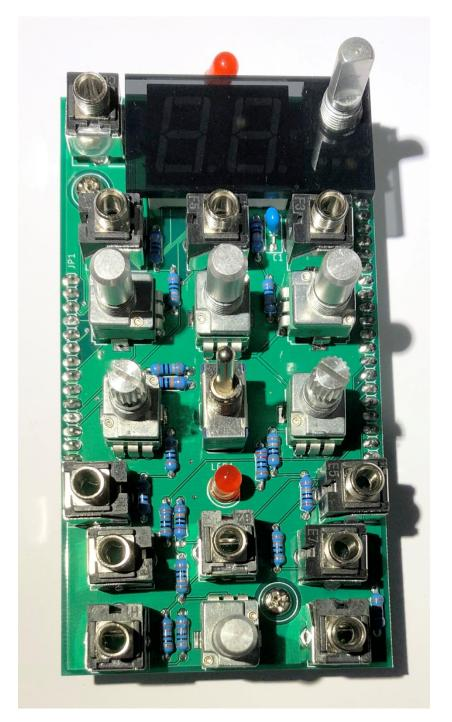
Place the panel back on. Place the nut for the SPDT switch on and finger tighten.
