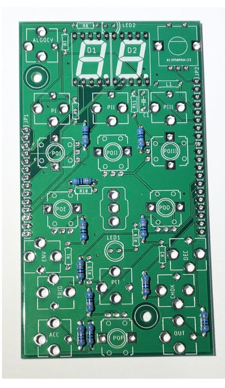
Install and solder the six 200K resistors R1, R2, R7, R9, R10, R11
