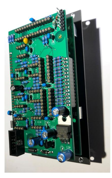
When the boards are connected and everything is sitting nicely, solder the remaining pins of the pin header.
