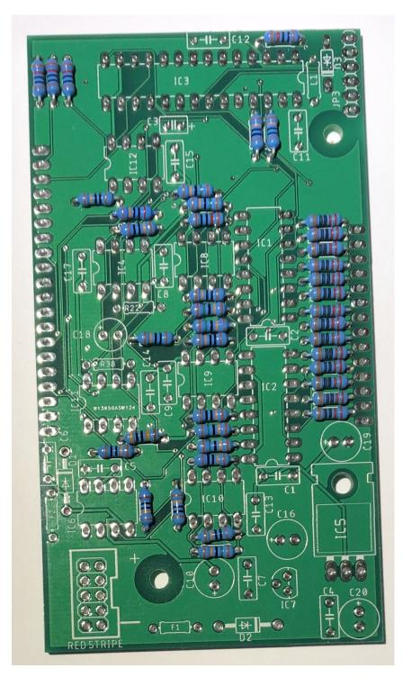
Install and solder the two 1M resistors R22 and R38
