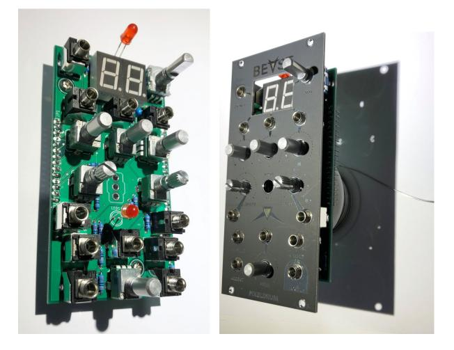
Carefully place a washer and nut on the PI and PIII pots. Also place two knurled jack nuts on the accent and out jacks. Very gently tighten the nuts until they are "finger tight" DO NOT over tighten them as they will twist the pots and jacks and/or pins will be bent.
