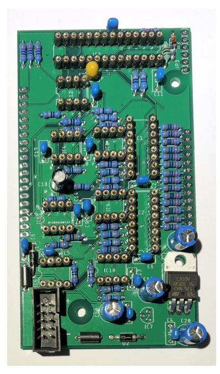
Install the 79L05 voltage regulator IC7. Make sure the flat side is facing the same direction as the silkscreen on the PCB.
