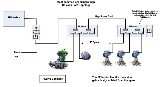
Segment with more than one coupler. Note the couplers can be mounted in junction boxes.
