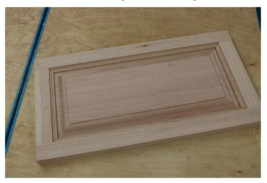
Assemble your door. Don't glue solid wood panels into the frame. This prevents them from expanding and contracting. Use Space Balls to prevent the panel from rattling in the frame.
