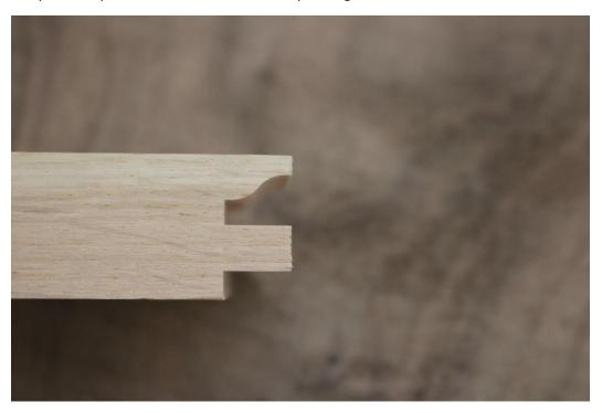
When the height of the end grain cutter is right, the lip on the front of the door should be about 3/32" thick, and the shoulder on the back about 3/16" deep. Save a correctly cut test piece and use it to set the height of the bit the next time you make doors.
