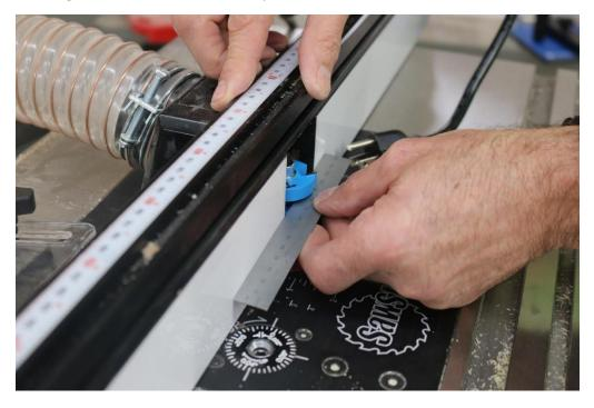
Position the fence by spanning the opening in the fence with a straight edge and aligning the fence with the ball bearing on the bit.
