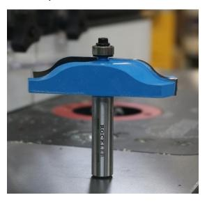
Before installing the large diameter panel raiser, lower the rpm of the router. Use the speed chart (Sources) to get the speed right.
