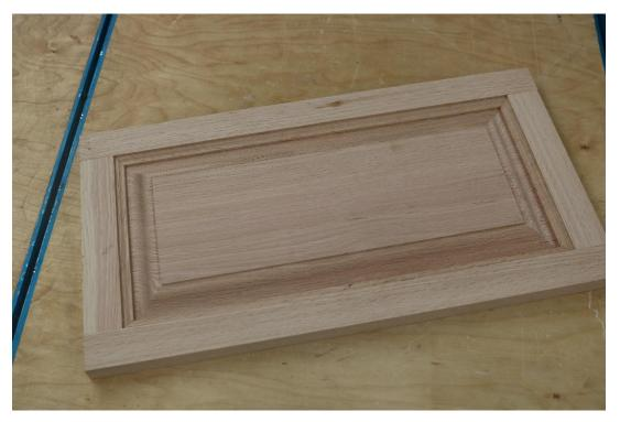
With the right set up and a few tricks, it's easy to make raised panel doors on the router table.
