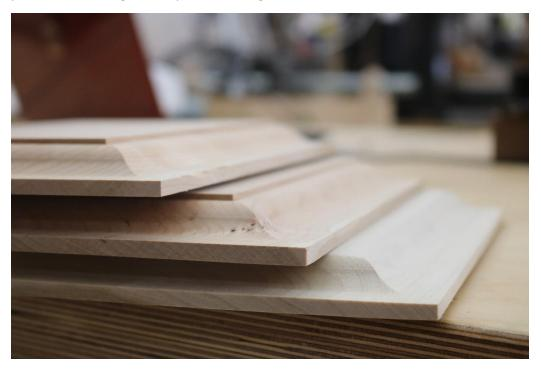
There are various approaches to raising panels. If the panel is the same thickness as the frame you will probably need to cove cut the back side of the panel; top panel here. If the panel is thinner than the frame you can skip the back cut.
