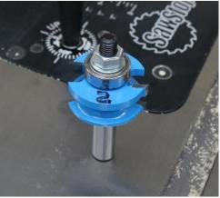
Using a felt tip marker draw a number 1 on the end grain cutter, and a 2 on the long grain cutter to remind you that you'll always use the end grain cutter first.
