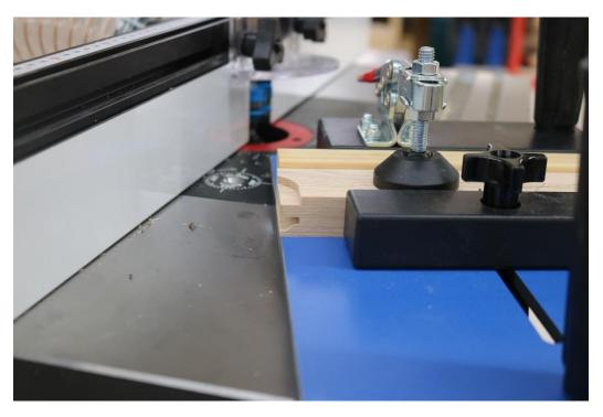
Cut your test piece, but don't cut all the way through it and into the backer.
