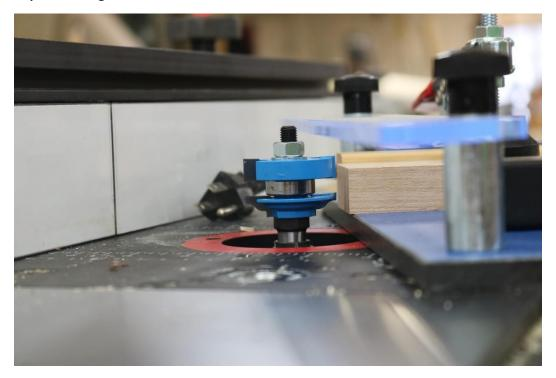
With a test piece in the coping sled, set the height bit number 1, the end grain cutter. Set this by eye, shooting for a balance between the lip on the front of the rails and the shoulder on the back.
