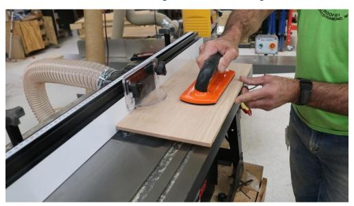
Raise the panel, making multiple light passes, with the marked face up. Cut in this sequence; end grain, long grain, end grain, long grain. This sequence allows the long grain cuts to clean up any chipping on the exit side of the end grain cuts. Raise the bit, make another pass, raise the bit make another pass....until the edge of the panel fits the groove in the frame.
