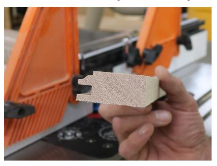
On many cope and stile sets the shoulder on the front of the frame aligns with the groove in the frame. This makes it easy to measure for panels. Dry fit the door and measure from shoulder to shoulder.
