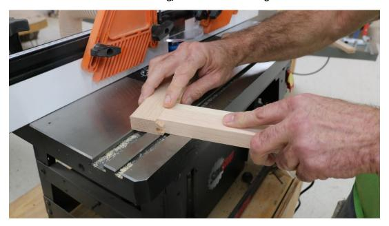
When the height of the long cutter is right, the face of the rail will align with the face of the mating piece. Don't worry about making it absolutely perfect. If there's a slight "fingernail catch" between the faces don't sweat it. It'll easily sand off later. When the height is right, do the long grain cut on all your door parts, keeping the marked face up.
