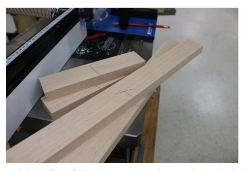
Mark the back faces of all your door parts. Using the coping sled, machine both ends of all the rails with the back, the marked face, up.
