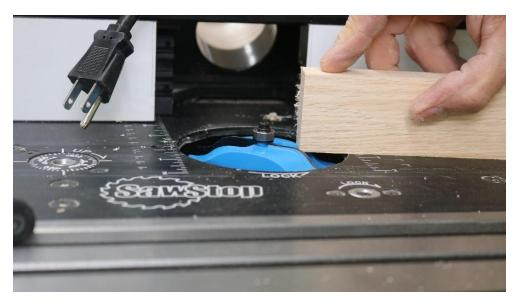
Set the height of the bit so its highest point is 1/8" above the table surface. Use a block of wood as a straight edge to gauge this.
