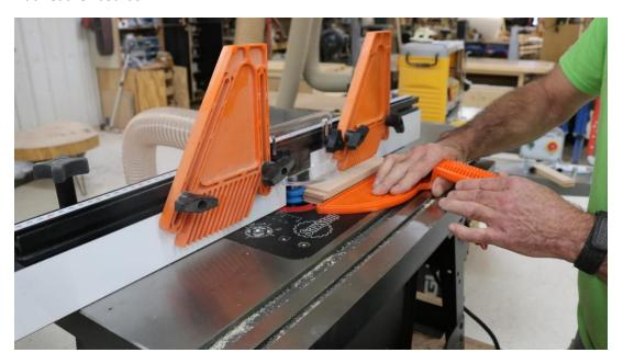
Cut a test piece and check your work. Use a push stick that allows you to put horizontal pressure, not vertical pressure, on the pieces. This helps prevent them from tipping and ruining the cut, especially on long pieces.
