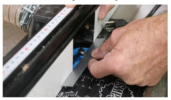
Make the face of the fence even with the ball bearing on the router bit.
