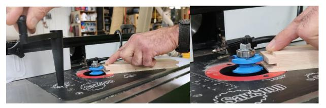
Install cutter number 2, the long grain cutter. Set its height by making the top of the carbide on the groove cutter even with the top of tongue on the end of the rail.
