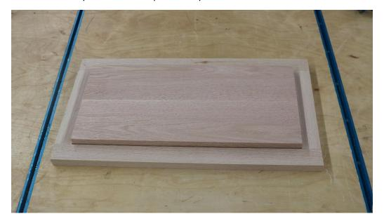
If your panel fits in the shoulders on the front of the frame, it'll fit in the grooves. Mark the back face of the panel.
