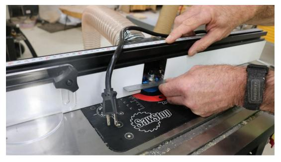
Make the face of the fence even with the ball bearing on the bit.
