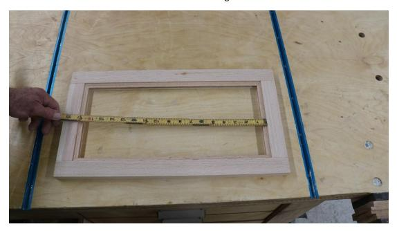
Measure for the panel. The panel should be smaller than the groove to groove distance to allow for expansion and contraction.
