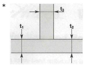
Combined Plate Thickness: T Joint:  $t = t_1 + t_2 + t_3$ Butt Joint:  $t_3 = 0$
