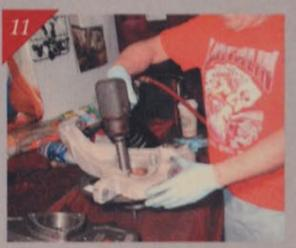
At this juncture, Richard uses an air impact gun equipped with a 15mm socket to remove the hub assembly from the Dodge factory aluminum spindle.
