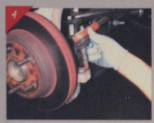
Next, Richard uses an air impact gun to remove the passenger-side tie rod end using a 21mm socket.
