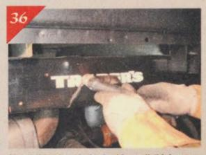
Since this chassis is double wall thickness, it only makes sense to use a plasma cutter. Sure, you can use a smoke wrench. That is IF you want to take all day to do the job!
