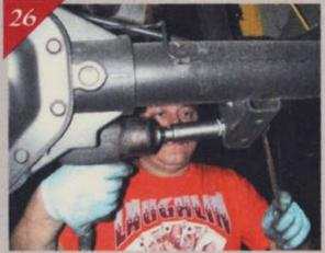
Pineda kicks things off in the rear by removing the lower 21 mm shock bolt from the passenger side of the truck.
