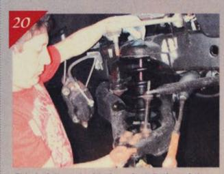
This is followed with the reinstallation of the factory Mopar front shock using the 1/2-inch factory shock absorber retaining nuts.
