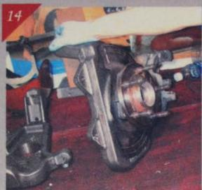
Reassembly begins with the installation of the Mopar factory hub carrier onto the McGaughy's dropped front spindle assembly using the OE 15mm factory mounting bolts.
