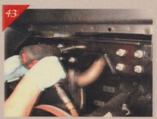
And finally, our installer bolts together the entire assembly using the 7/16-inch nuts provided. These nuts are final-torqued to 75 lb.-ft.
