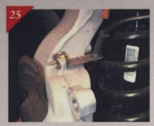
Also shown is the location on the driver's side spindle where the ABS brake sensor line mounts up. This has to be removed before removing the actual spindle/hub carrier assembly. A new provision is drilled into the new spindle. Other than this, the changeover is the same as the passenger side.
