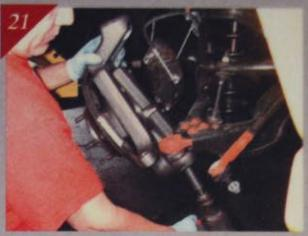
Reinstallation of the new McGaughy's ductile iron dropped front spindle assembly comes next and is bolted into position using a 21mm socket.
