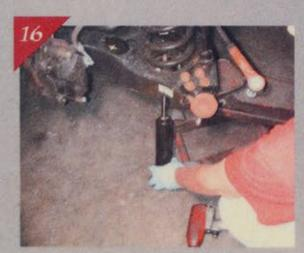
Pineda removes the factory shock absorber, which will also be reused.
