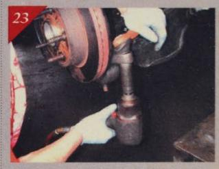
This procedure is followed with the reinstallation of the factory tie rod end using a 21mm socket.
