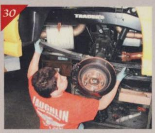
With U-bolts removed, Pineda removes the passenger side leaf spring from the truck, while a floor jack supports the rear end.
