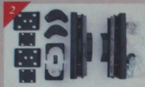
Shown is McGaughy's Suspension Parts' 4-6 deluxe drop kit for the 2002-04 Dodge Ran 1500 light duty truck line. Included in the deluxe kit (P/N 02D-46D) is a pair of McGaughy's CNC-machined, ductile-iron dropped front spindles (patent pending); a pair of progressive wound, 1,500-pound lowered front springs; a rear flip kit, which includes the correct pinion angle design spring locator brackets; rear shock extender brackets; McGaughy's design bump stops; and C-notch kit.
