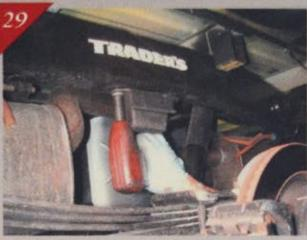
Next comes the removal of the factory bump stops, using an air gun and a 15mm socket.
