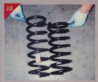
This comparison photo clearly shows the difference between the factory spring on the left, and the McGaughy's spring on the right. However, the spring rate (1,500 pounds) remains the same.
