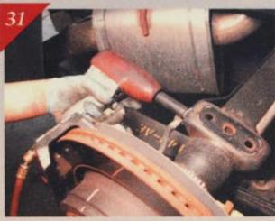
The next order of business is the removal of the Dodge brake line bracket from the rear axle using a 13mm socket.
