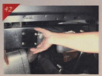
Since there is a step in the factory frame, McGaughy's also provides a shim plate, which we see being installed here.
