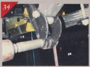
Next comes the reinstallation of the factory shock onto the McGaughy's shock extender bracket using a 21mm socket.
