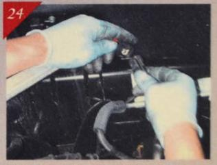
Moving over to the driver's side, Richard begins by removing the ABS brake sensor wire from its retaining clip located at the bottom of the fender well.
