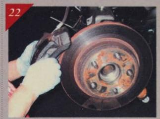
With that done, the next order of business is the reinstallation of the disc brake rotor and caliper assembly using the factory 18mm bolts.
