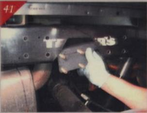
At this juncture, Pineda test-fits the inner support bracket, sliding it up inside of what remains of the Dodge Ram 1500-Series rear frameralls.
