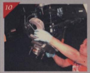
And out comes the actual spindle assembly itself with hub carrier still attached.
