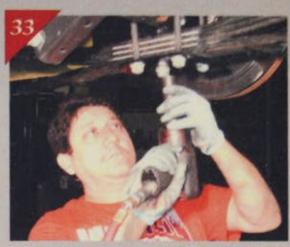
With saddles in place, the factory U-bolts are reinstalled with McGaughy's spring plate and 21 mm U-bolt nuts.
