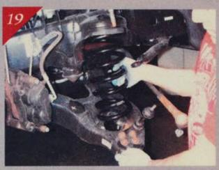
Reassembly begins with the installation of the McGaughy's spring into the spring saddle using the factory rubber insulator.
