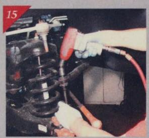
Next, Richard removes the anti-sway bar end link using a 15mm socket.
