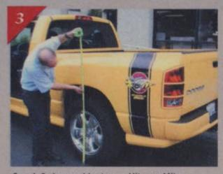
Our 4-6 drop subject was Nitrous Mike Golightly's yellow, 5.7L, 2004 Dodge Ram 1500 Rumble Bee Hemi pickup. Prior to unbolting anything, Golightly measures the ride height front and rear, and comes up with a measurement of 16 1/8 inches front and 39 inches rear.
