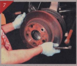
After removing the safety clips, which retain the front disc brake rotors in place, the actual rotor itself is removed.
