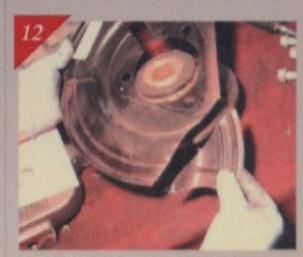
With this kit, it's necessary to trim the front tip of the dust shields in order to clear the revised tie rod end geometry following the illustrated instructions provided in the kit.
