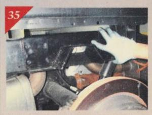
in this photo, Pineda uses the opposite side C-notch bracket to make a template (using spray paint) onto the Rumble Bee's rear framerail. Since this area will be cut, Richard double and triple checks his marks.
