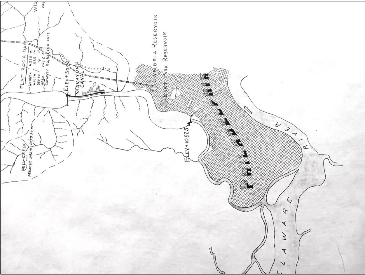
Flat Rock Dam # 31 and Lock 68 begins the Manayunk Canal, ending at Locks 69-70; and a short canal called Fairmount began with Guard Lock 71 and ended at Tide Lock 72 below Fairmount Dam # 32.
