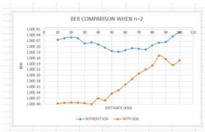
Figure 14 BER Comparisons with and without SOA for n=2 and d=10 Km to 100 Km
