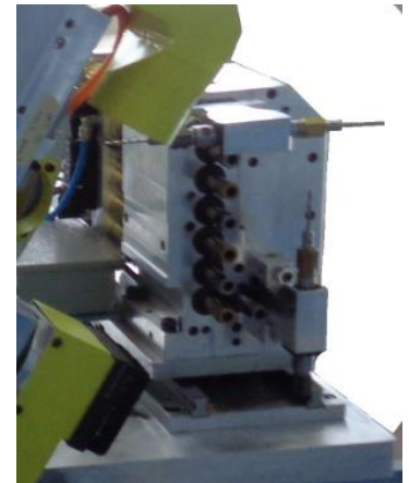
Independent Boring Unit on the Back Side of the Bridge
