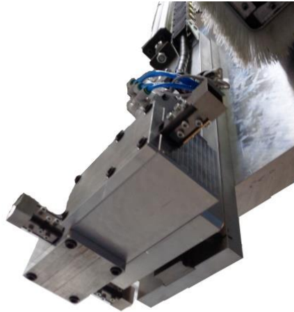
Square Chisel Unit on the Back Side of the Bridge
