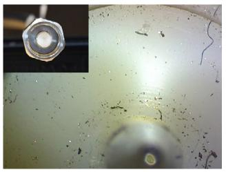
The N-Connector in the small image top left looks clean with bare eyes. The view though a microscope reveals however many alien bodies that can be a serious source of passive intermodulation distortion.
