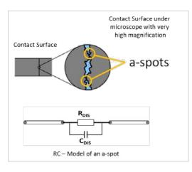
Structural material discontinuity causes also discontinuity in current flow. Regardless of the contact material, discontinuity in electron flow is characterized by:
