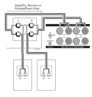
The other method is to connect the amplifier to the main speakers and then run extension wires from the main speakers to the ICS Sub 24.
