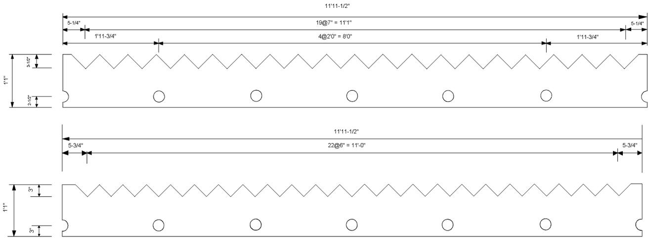
The sizes of weirs & baffles indicated are sizes that are available as standards in molded or pultruded weirs and baffles. In pultruded weirs any size and notch configuration may be furnished. In scum baffles there are many more pultruded options available up to 4' tall scum baffles in flat plate and reinforced baffles as indicated below.
