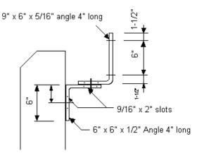
Fiberglass Scum Baffle Alternate Support Brackets Angle sizes can be interchanged, sizes that are available are:
