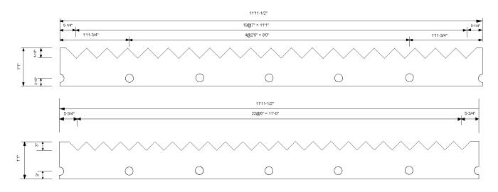
The sizes of weirs & baffles indicated are sizes that are available as standards in molded or pultruded weirs and baffles. In pultruded weirs any size and notch configuration may be furnished. In scum baffles there are many more pultruded options available up to 4' tall scum baffles in flat plate and reinforced baffles as indicated below.
