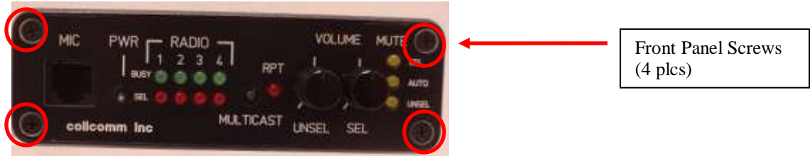
Front View of Unit –Note the four (4) mounting screws
