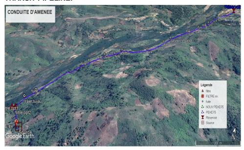
The total length of the supply pipe is 2,360 meters in PEHD D75 (75mm PVC). There were pipeline leaks detected during the field visit.
