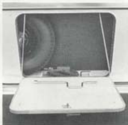
Rear Trunk, Spare Tire Storage
