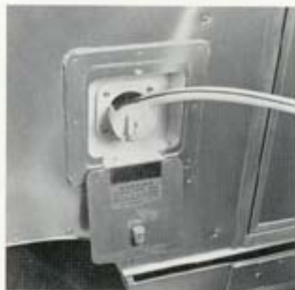
Water Tank Fill Spout
