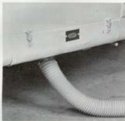
Sewer Hose Connection (in a Park)
