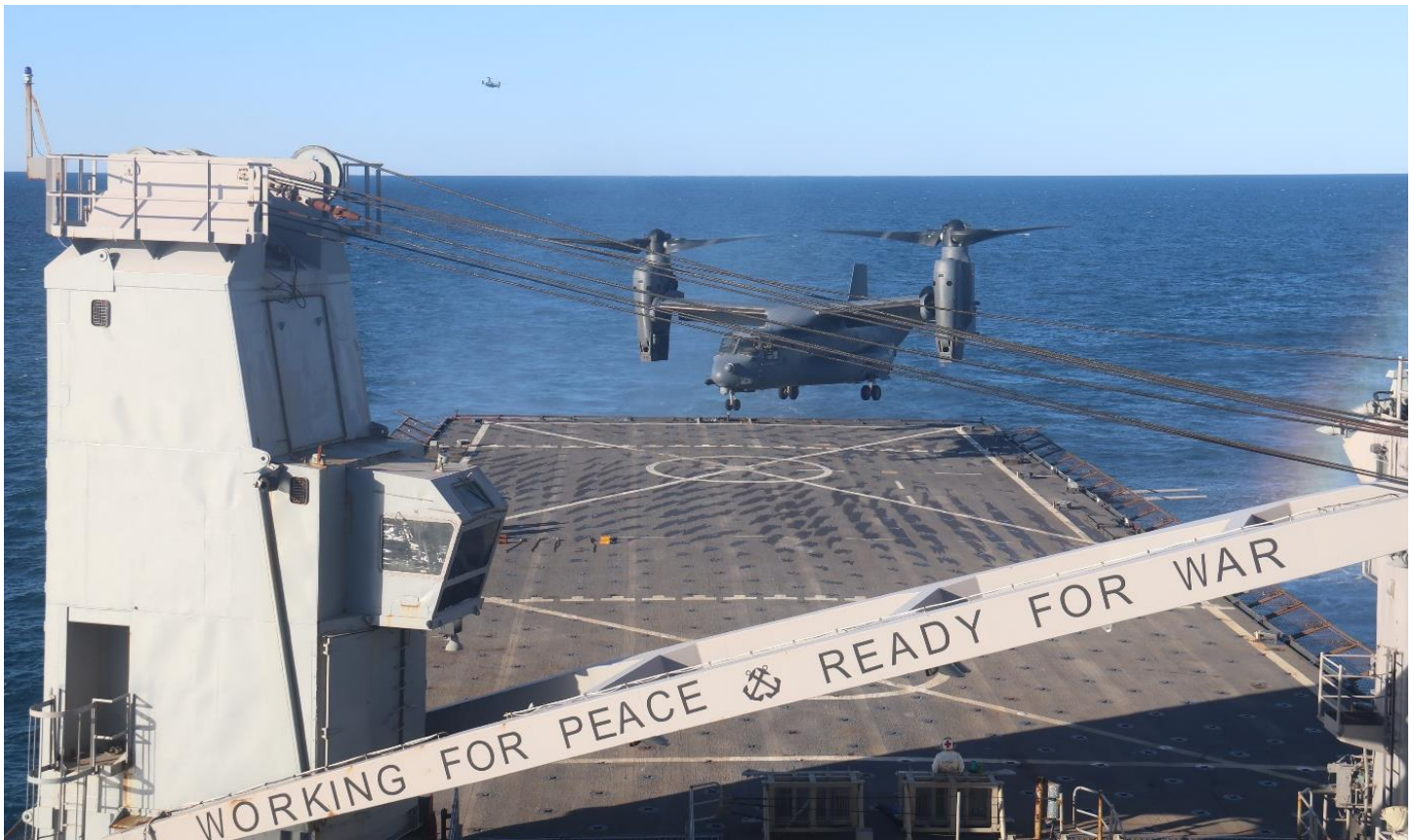
USS CARTER HALL conducts flight operations with a CV-22 Osprey. The Osprey is a multi-mission, tilt-rotor military aircraft that, with a crew of four, can carry 24 combat equipped troops or 20,000 lbs. internal or 20 lbs. external.
