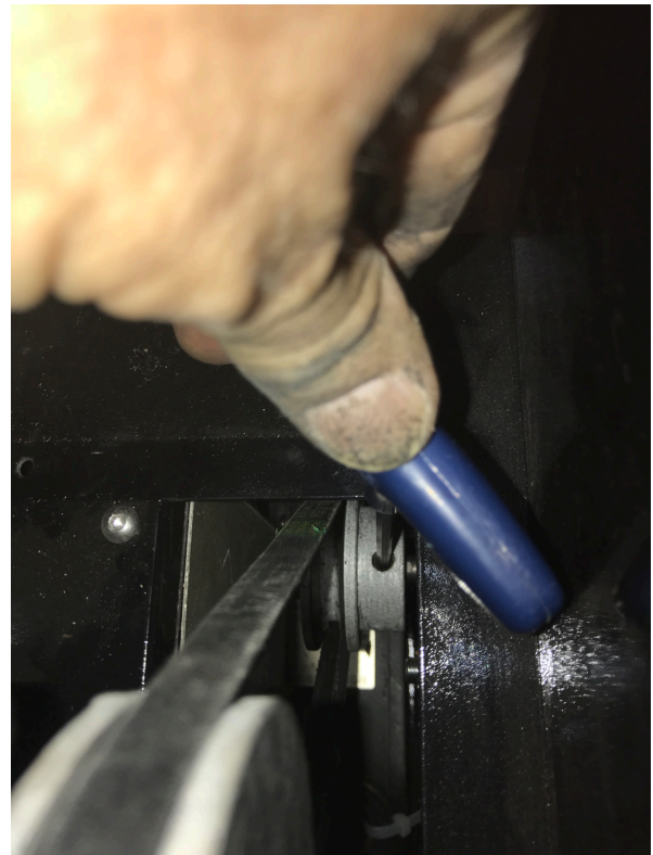
LOCATE HEX KEY PIN ON PULLEY AND LOOSE.
