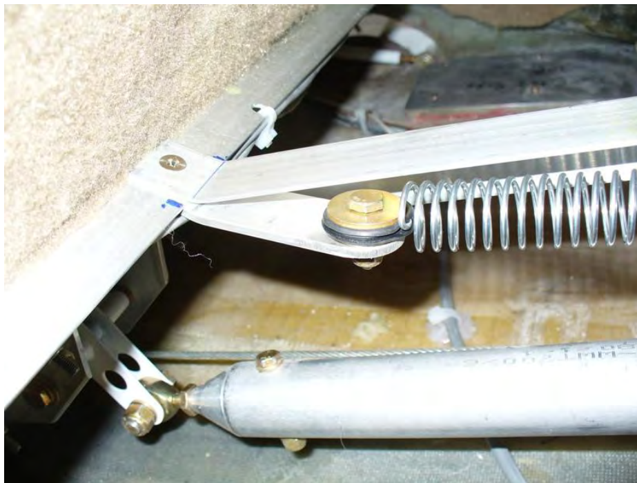
Other end of elevator assist spring secured to the seat back.
