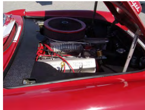
Vette's engine is a blown 383 putting out 575 HP.
