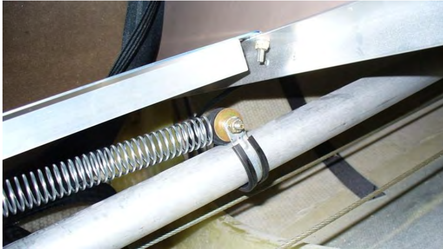
Elevator spring assist attached to the elevator push – pull tube.
