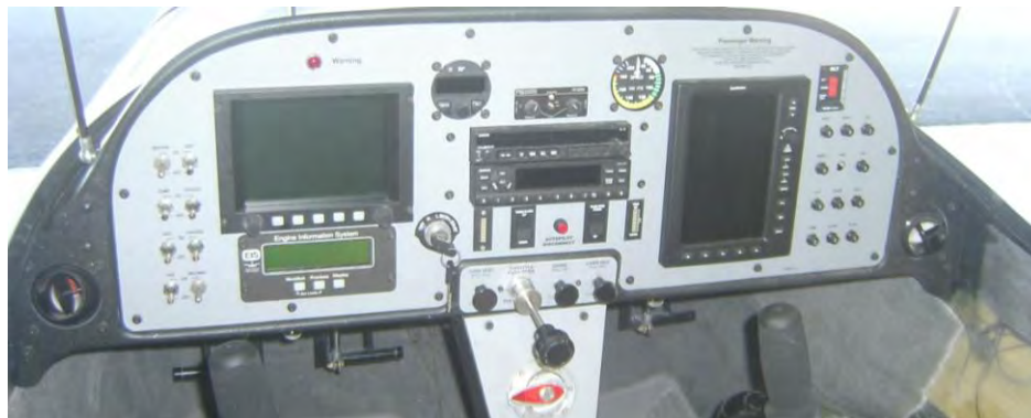
Panel of N326AL with Garmin GDU375 on the right side.
