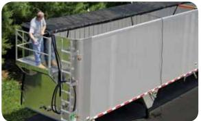
• Front Hand Crank opens the tarp system from the front catwalk (catwalk and ladder not included)
