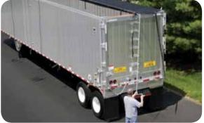
• Gound-Level Rear Crank manually rolls tarp system open or closed at rear of trailer from ground level
