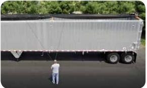
• Attached Full Rope Pulls allow tarp system to be pulled closed from the ground eliminating the need to crank
