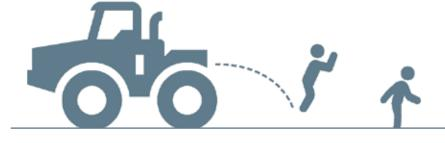
Hop or shuffle away from an energized line until you are 10 meters (33 feet) away
