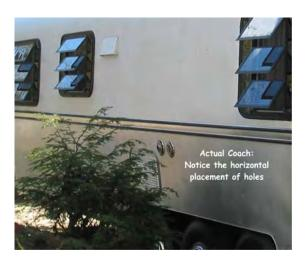
Our extensive study of replacement furnaces told us that the new furnace would use a vertical hole arrangement; therefore, our existing horizontal holes would not be useable. For safety reasons, the manufacturer strongly warns that intake and exhaust tubes NOT be bent or shaped, but should be connected directly to the holes in a straight line. We'll take their advice on that one, too!
