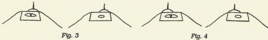
Sight adjustment for gun with back sight
