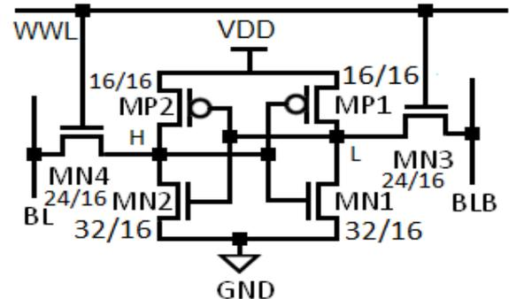
Figure 2: Standard 6T SRAM cell (D6T).
