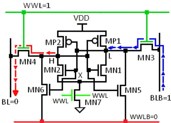
Figure 5: Write Operation of the proposed 8T SRAM cell
