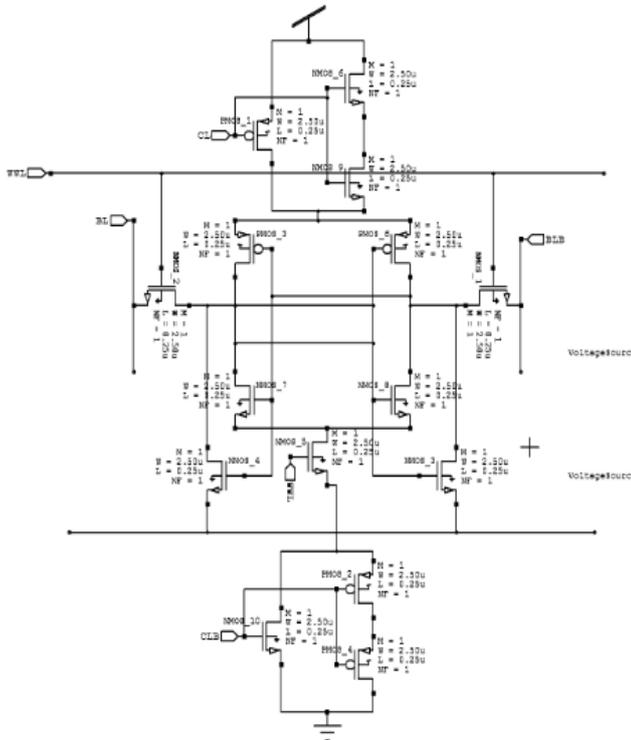
Figure 8: SVL Based 8T low Power SRAM
