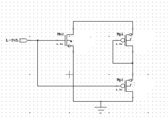
Figure 7: Lower SVL Circuit
