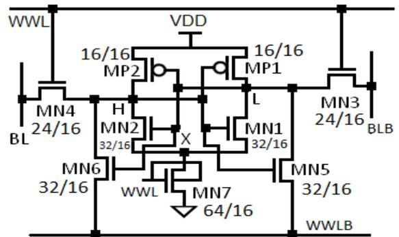
Figure 1: Low Power Consuming 8T SRAM cell (LP8T).
