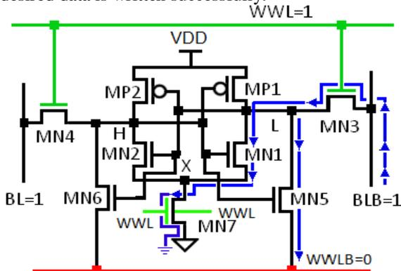
Figure 4: LP 8T SRAM cell
