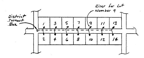
According to the attached head loss table, 21/2-inch pipe is required for a velocity of less than 5-feet-per-second-between the District's delivery box and the risers for lots 9 and 10. Two (2) inch pipe may be used beyond that point. (See attached.)
