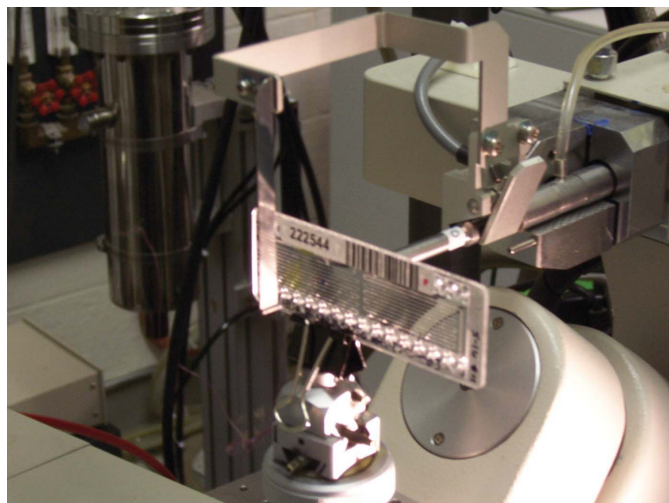
Figure 4 Picture of a CrystalCard mounted on a goniometer for in situ diffraction experiments.
