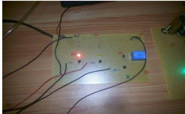
Figure 6: Yellow LED- Level 2 reached Indicating the tank is half filled
