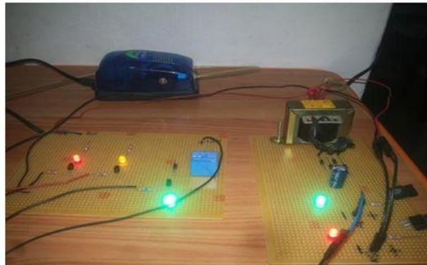
Figure 7: Green LED- Level 3 reached indicating the tank is completely filled
