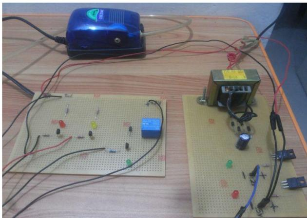
Figure 2: Hardware Kit Setup (PCBs with necessary components, Motor & Power Supply)
