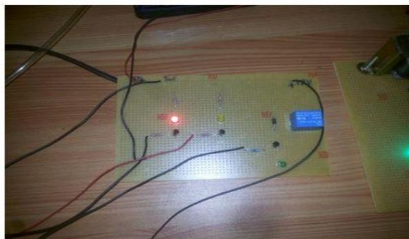
Figure 5: Red LED- Level 1 reached indicating the tank is slightly filled
