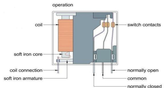
Figure 3: SPDT Internal Structure
