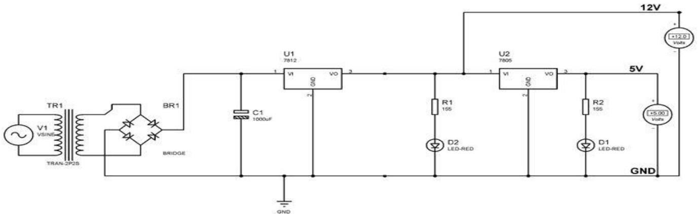
Figure 4: Circuit Diagram of Dual Power Supply of 12V and 5V
