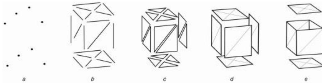
Fig. 3 Mesh representation of a 3D object (or polygon mesh representation) (a) Vertices, (b) Edges, (c) Faces (d) Polygons, (e) Surfaces [67]
