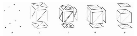
Fig. 3 Mesh representation of a 3D object (or polygon mesh representation) (a) Vertices, (b) Edges, (c) Faces (d) Polygons, (e) Surfaces [67]
