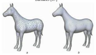
Fig. 4 Triangle mesh and quad mesh of 3D horse (a) Triangle mesh, (b) Quad mesh
