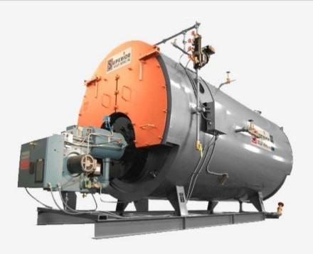
The Ohio Special is designed for maximum efficiency, reliability and durability in today's most demanding environments. All Ohio Special boilers have less than 360 square feet of ASME heating surface. Designs include a 2 or 3-pass dryback and a 3-pass wetback with pressures of 15 to 300 psi steam and 30 to 160 psi hot water. Boilers are available in sizes ranging from 80 to 225 BoHP.
