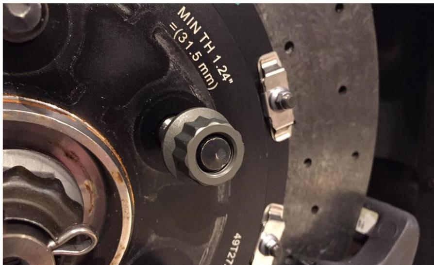
*Lug nut installed on a Viper ACR (without wheel)*
