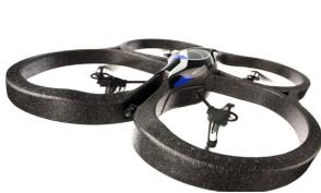
Figure 1.16: Parrot AR Drone with indoor hull [14]
