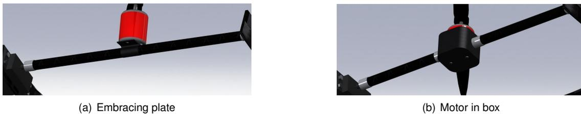
Figure 2.3: Possible motor connections for the U-arm
