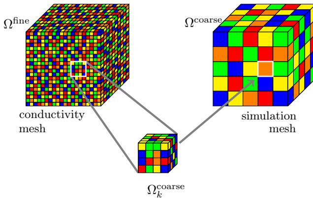
**Figure 1:** A fine conductivity mesh (left), a nested coarse simulation mesh (right) and one coarse cell with nonconstant  $\sigma$  (middle).
