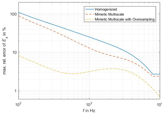
**Figure 4:** Maximum relative data error with respect to the reference solution on the fine grid for electric fields  $E_x$  recorded at 31 receiver locations.
