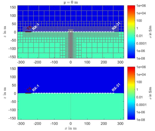
**Figure 2:** Vertical borehole in a homogeneous half-space: with mesh (top) and without (bottom).
