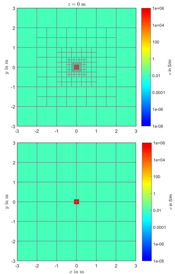
**Figure 3:** Borehole in plan view: fine conductivity mesh (top), coarse simulation mesh (bottom).
