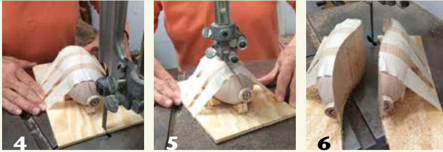
4 The author's pod cut in half on a curved line. The tenons at each end can be cut off after the pod is split. 5 6
