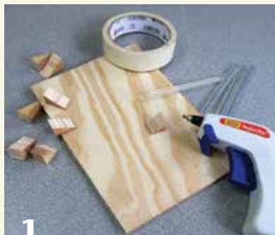
1 Materials needed: scrap wood, wedges, hot-melt glue gun, glue, and masking tape.
