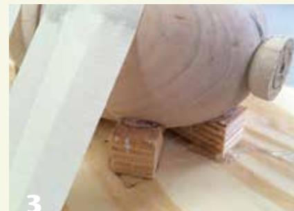
2 Workpiece is glued and taped to the wedges and carrier, ready to be cut apart on the bandsaw. Note the intended cut line for this pod form (along the sidegrain). The jig can also be used to cut across the grain to remove a tenon.
