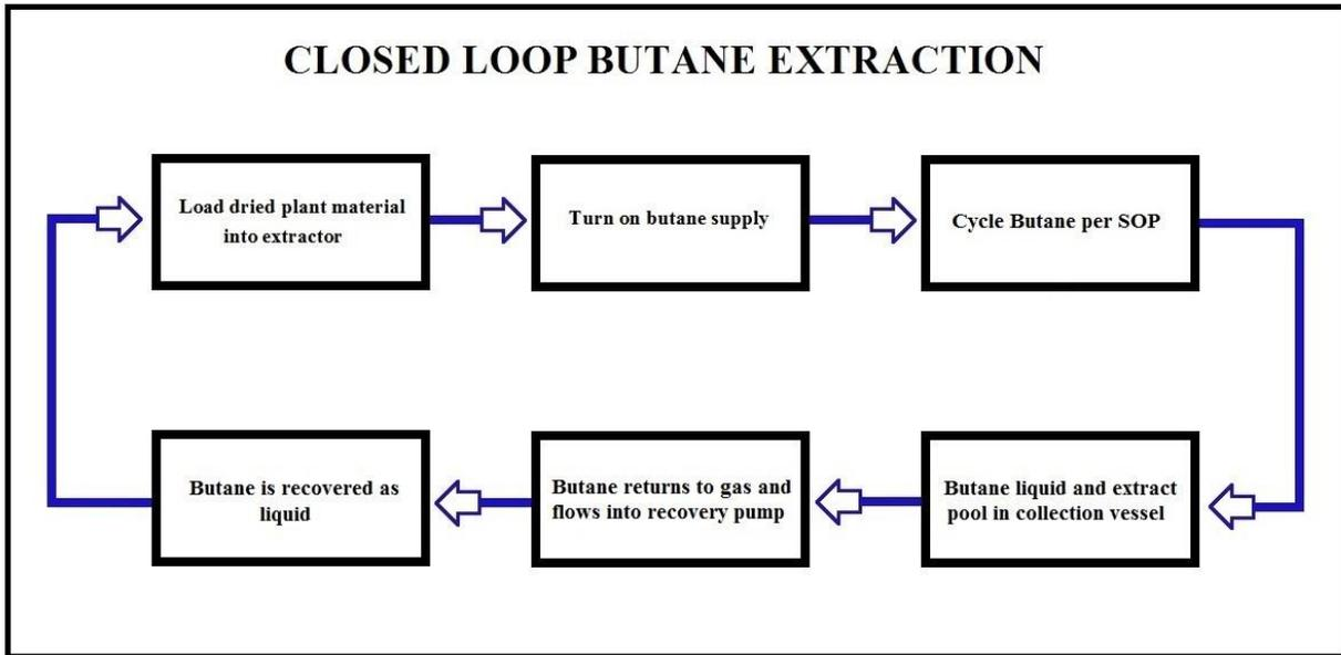
Figure 1: Butane Extraction System Flow Chart
