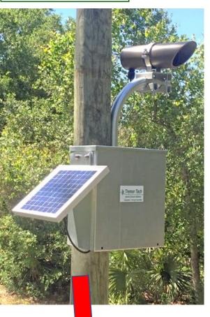
The TTech-81PIR Curtain Sensor has the ability to generate an invisible detection zone which will activate when subjects and objects are detected passing through it.
