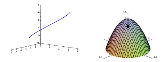
We now do the same except instead of a line, we do this with a surface. Assume that the density of a surface is given by  $\rho(x,y,z)$ . The shape of the surface is given by S(x,y,z). If we have a small part of the surface, denoted by dS, then the mass of the little part of the surface is  $\rho(x,y,z)dS$ . Now add up the little pieces and in the limit we get
