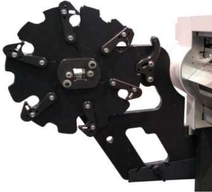
2. Repeat Step 1. For the Left Side Rotating Wheel, again ensure that the wheel faces the inside of the machine.
