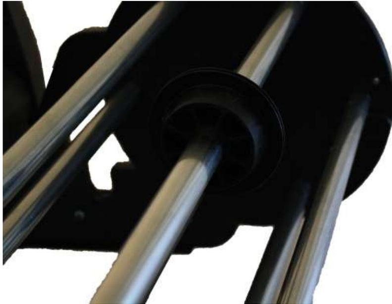
8. Slide the desired film or vinyl onto the Chrome Tube with a Cone on each end and tighten the set screw with the 1/8" Coated Hex Key. Once you have determined your desired location for the Cones so that your material is lined up with your plotters' feed rollers, you will seldom need to adjust the position of the Cones on the right side of the Chrome Tube. At this time, simply remove the left Cone and exchange your media (film or vinyl). Reinstall the left Cone and no realignment is necessary.
