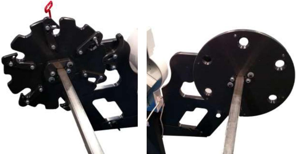
6. At this point you may have noticed that the Right Side Wheel has an extra piece attached to the outside of it. This piece is a holder for the included 1/8 Coated Hex Key. There is also an extra hole for another plotter blade (not included). Place the Coated Hex Key in the holder.
