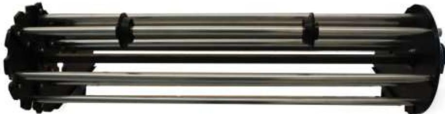
11. Your Fusion Revolver is now completely assembled. You can pull the lever on the Right Side Wheel and rotate the Wheels to the desired film or vinyl choice and begin cutting. **To ensure a properly balanced machine, it is recommended that you keep all 6 chrome tubes mounted with the media of your choice.**
