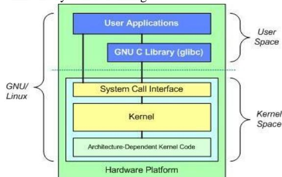
Fig.4: Architecture of Linux Operating System
