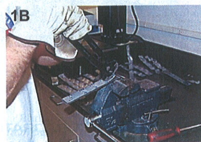
Fig. 1 — Destructive testing methods for resistance spot welds on thin sheet metals: A — Drive test; B — peel test.
