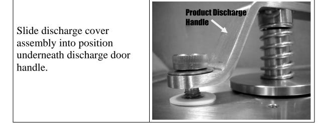
Press down on product discharge handle, ensuring the discharge cover and discharge handle are aligned with each other.
